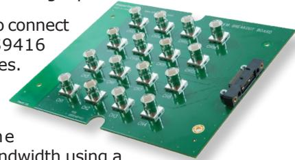
As mentioned in the *Wideband Input Upgrade* section, the maximum achievable bandwidth using a breakout board and QSS-QSS cable is 10 MHz.
