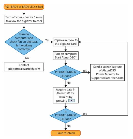
Figure 4 - Flowchart for Power Monitor Status LEDs
