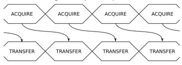
Figure 6 - AutoDMA acquisition and transfer cycle
