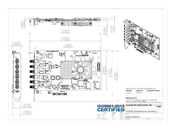
Figure 2 - ATS9352 Mechanical Drawing
