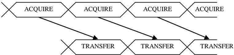
Of course, software still has to set up the DMA when one of the buffers fills up, but, thanks to the dual-DMA engine and fully asynchronous driver that uses overlapped IO, these tasks can be paralleled.
