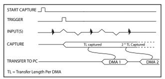
Triggered Streaming AutoDMA buffers do not include headers, so it is not possible to get trigger time-stamps.
