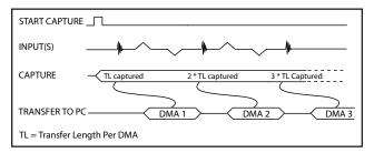
In this mode, data starts streaming across the PCI bus as soon as the ATS660 is armed for acquisition. It is important to note that triggering is disabled in this mode. Continuous AutoDMA buffers do not include headers, so it is not possible to get trigger time-stamps.
