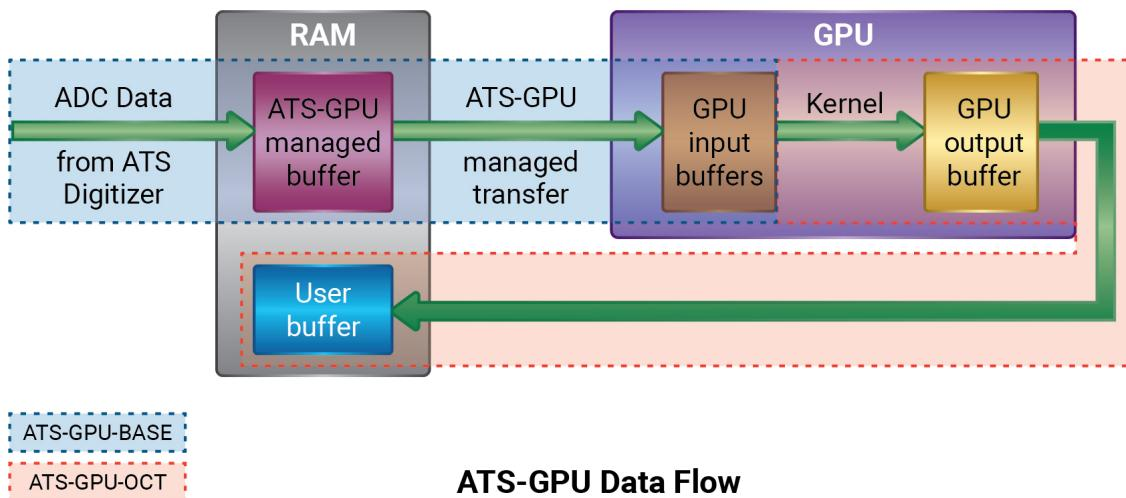
The **ATS-GPU-OCT** add-on library provides out-of-the-box OCT imaging. It consists of a library of CUDA kernels that operate on the data acquired by **ATS-GPU-BASE**. Up to 950,000 4K FFTs per second can be calculated, which is more than sufficient for existing swept sources on the market. Windowing, Zero Padding, Dispersion Compensation, and Log functions are also included.
